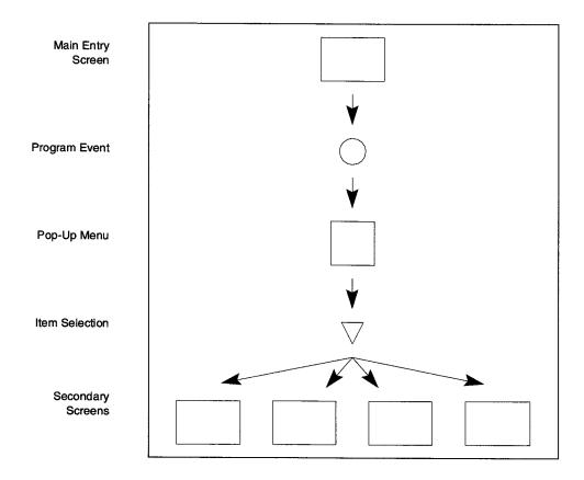
Recall from chapter 11, you used the <code>switchbox\_items</code> trigger, the <code>fgStack\_push()</code>, and the <code>socketManager()</code> function to attach an add-on header screen to your main screen. To attach secondary screens to a pop-up menu, you follow much of the same process. But you should note that different secondary screens are attached in different ways. At this point, you've only looked at add-on headers and zooms (and zoom screens are attached automatically).
