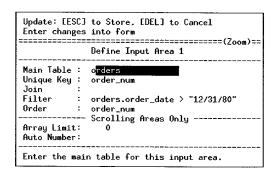
When you define the header input area, you cannot enter the Join field. This field is only for detail input areas.
