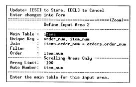
For a header/detail screen, you must specify characteristics about the detail portion of the form in order for the form to work properly. For instance, you must specify the join that connects the header table to the detail table.
