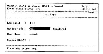
The most important field is the **Action Code** field. This field corresponds to the Action Code you gave the event in the Navigation Commands window (page 9). The System Wide? field specifies if the Hot Key is available to all system users.
