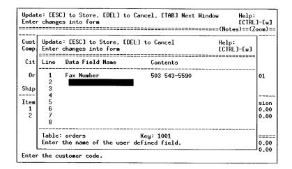
User-Defined Fields are not physically entered into a column on the header or detail table. A separate table stores these field labels and contents. If users define a number of fields, you should consider adding those fields to the input program with the Form Painter.
