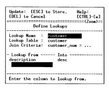
If the fields and columns have the same name, you do not need to add them to the Lookup From and Into fields. The *Screen* Generator builds this logic when the field names and column names match.
