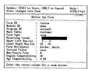
Make sure to specify a value in the Returning (zoom) field. This field specifies where the returning value gets placed In most cases, this is the field in which you attach the Zoom If you are not sure of the field, press [CTRL]-[z] while to see a list of available fields
