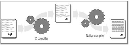
From the operating-system command line, a single call to the c4gl command performs all the steps, or all these steps can be automatically accomplished through the Progammer's Environment.
