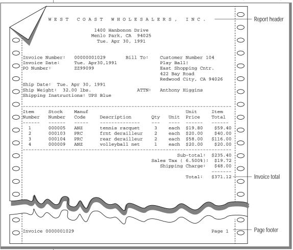
In 4GL, the program logic that specifies what data to report is separate from the program logic that formats the output from the report. Any 4GL program that produces output from a report must include a part that produces the data from a database (or from some other source), and a second part that formats the data as output from a report.
