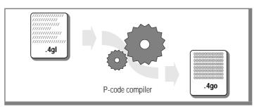
Figure 4-5 The P-Code Object Code Generation Process
